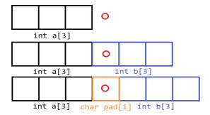
It worth mentioning that modifying allocators in such way introduce a problem when external code is involved, as the external code cannot be aware to the fact that memory was allocated in a different way, and will not use our customized allocators. In addition, changing sizes of objects passed as function parameters can change the memory layout of the parameters. Therefore, this workaround cannot be applied to objects and code that might be involved with external libraries.
