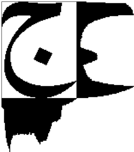
Figure 2.6: The vertical and horizontal black ink histograms of the letter \bar{j}im .
