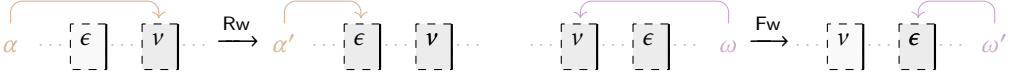
Fig. 12. Schematic depictions of the rewind and forward rewrite rule, focusing on a single location, where the initial/final view points to v before and points to \epsilon after. The messages v and \epsilon may coincide, dovetail, or be separated. Left: The initial view \alpha is “rewound” to \alpha' . Right: The final view \omega is “forwarded” to \omega' .
